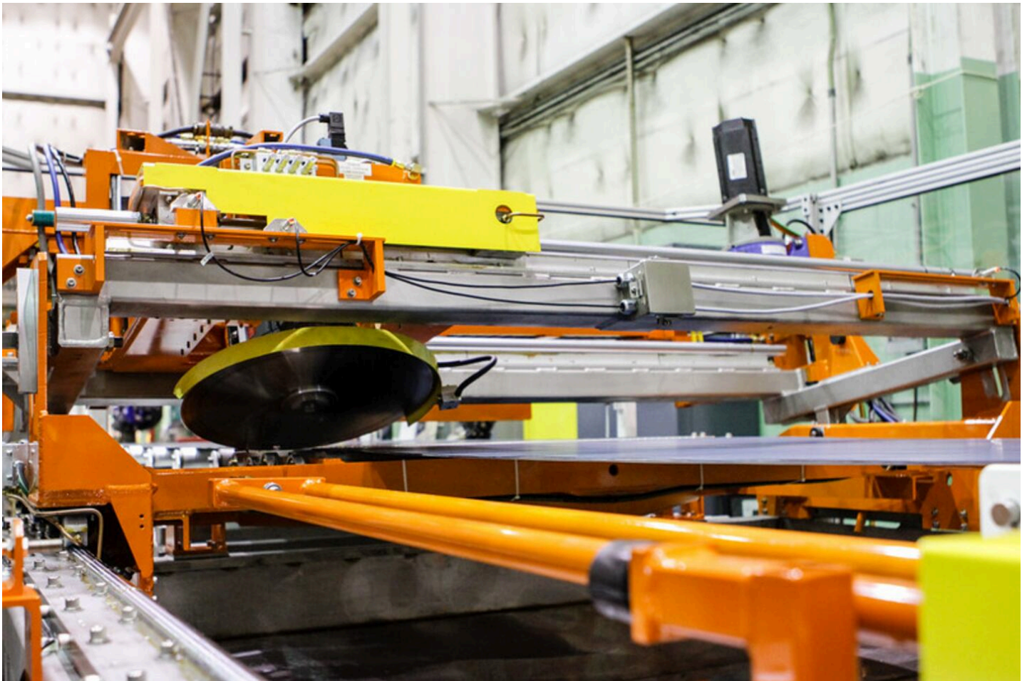
Spadone Skiver System-02_i.jpg Spadone Machine manufactures a variety of rubber equipment including bias cutters and this rubber skiver machines. (Photo courtesy of Spadone Machine)
